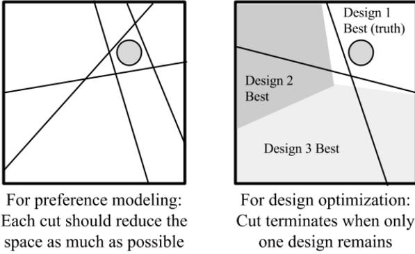
**FIGURE 2.** A comparison between adaptive questionnaire for preference modeling and for design optimization. The true preference model (the circle) is a point in a preference space (the square). Binary questions are cuts (the lines). With the profit model, the space is segmented, where segments are labeled by the corresponding optimal designs.
